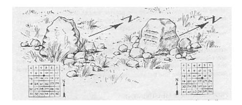
Marks on old stone section corners. The notches or grooves indicate the number of miles from the south and east boundaries of the township, respectively.
