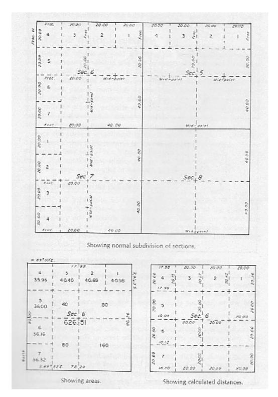
FIGURE 46, MANUAL Examples of subdivision by protraction
