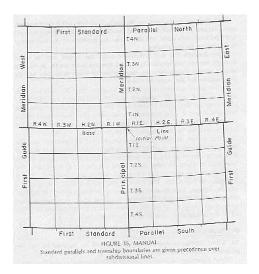
As between single or double proportionate measurement, the principle of precedence of one line over another of less original importance is recognized, in order to harmonize the restoring process with the method followed in the original survey, thus limiting the control.
