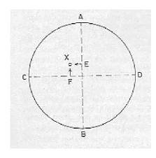
A, B, C, D,–Control corners E–Proportionate point for X in latitude between A and B F–Proportionate point for X in departure between C and D
