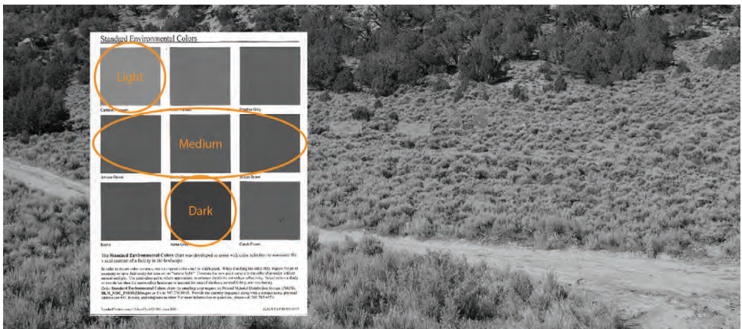
When choosing colors from the BLM Standard Environmental Color Chart for a two-color application, select one light tone and one dark tone. Patterns of three or more colors should also include mid-range tones.
