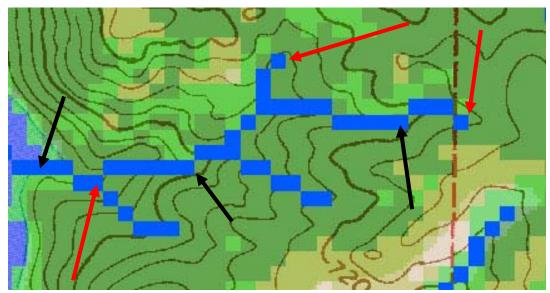
Figure 9 - Acceptable (black) and Unacceptable (red) Channel Cells
