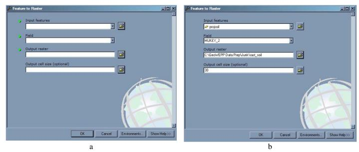
Figure 146 – a) The Feature to Raster tool parameter window; b) All parameters entered into tool
