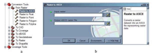
Figure 114 – a) Raster to ASCII tool in ArcToolbox tree; b) Raster to ASCII tool window
