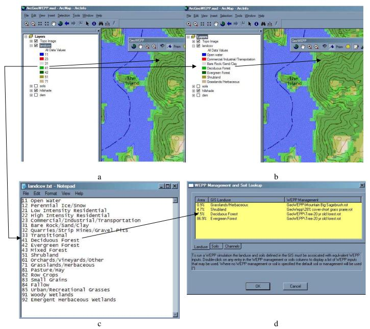
Figure 149 – Linkage between GeoWEPP, landuse text files and WEPP: a) GeoWEPP without legend descriptions; b) GeoWEPP with legend descriptions; c) landcov.txt; d) WEPP/TOPAZ Translator
