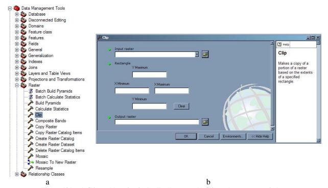
Figure 121 – a) Clip tool location in ArcToolbox tree; b) Clip tool parameter window
