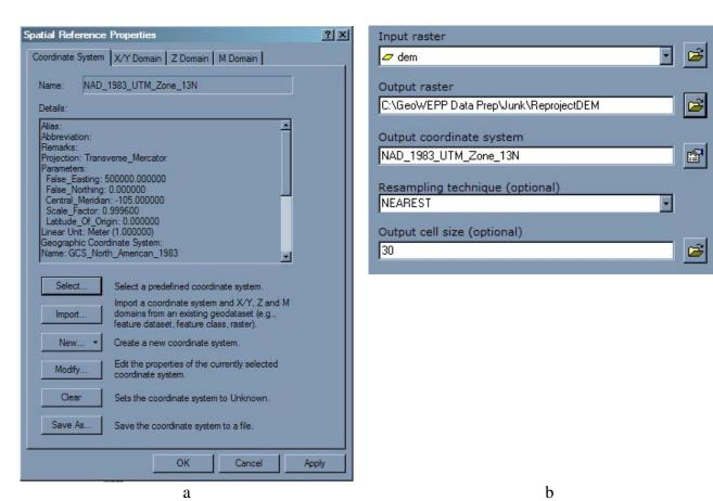
Figure 112 – a) Spatial Reference Properties window with UTM projection details; b) All parameters have been added
