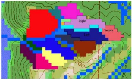
Figure 10 – Outlined Hillslopes flow into the light blue channel
