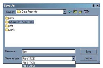
Figure 115 - Make sure the DEM is saved as an ASCII file
