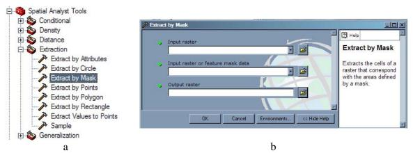
Figure 130 - a) Extract by Mask tool in the ArcToolbox tree; b) Extract by Mask tool window
