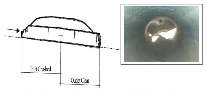
Length = 6' if pipe is larger than 24" diameter; replace entire length of pipe if diameter is 24" or less
