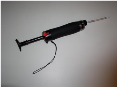
Sorbent Tube for Collecting Vapors
