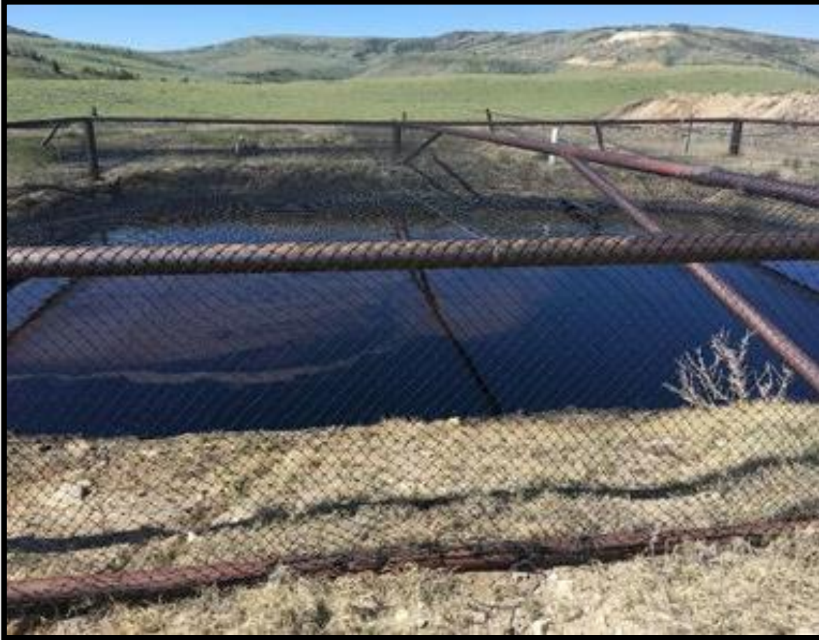
Oil covering fluids in the entire disposal pit
