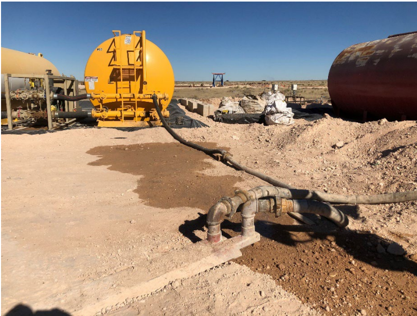
Active leak of produced water on NE corner of well pad
