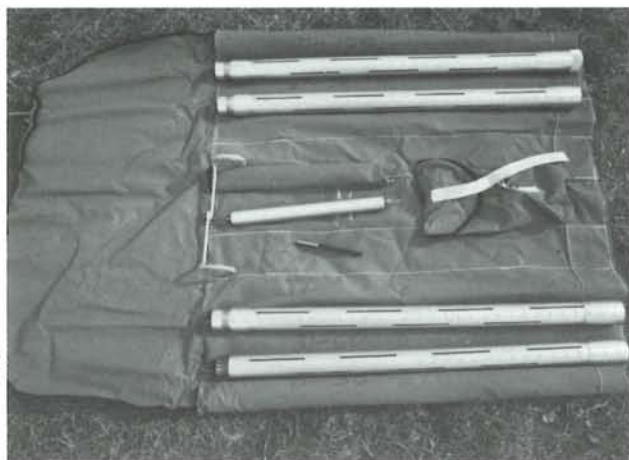
Figure 3. A standard federal snow sampler kit for measuring snow depth and water content.
