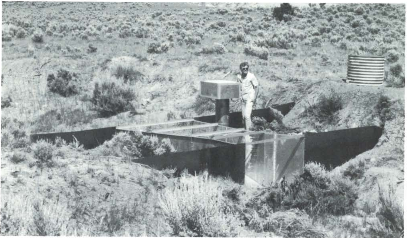
Figure 8. A Parshall flume for the continuous measurement of streamflow.
