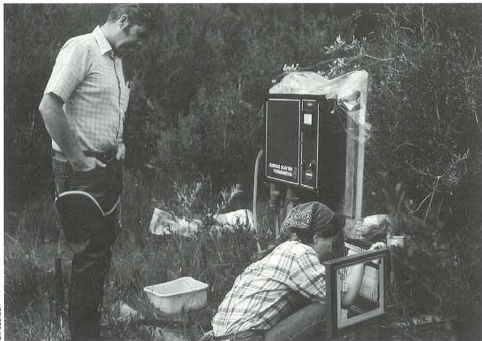
A surface scatter turbidimeter being used to monitor stream turbidity during a controlled reservoir release designed to flush fine sediments from the stream bed.
