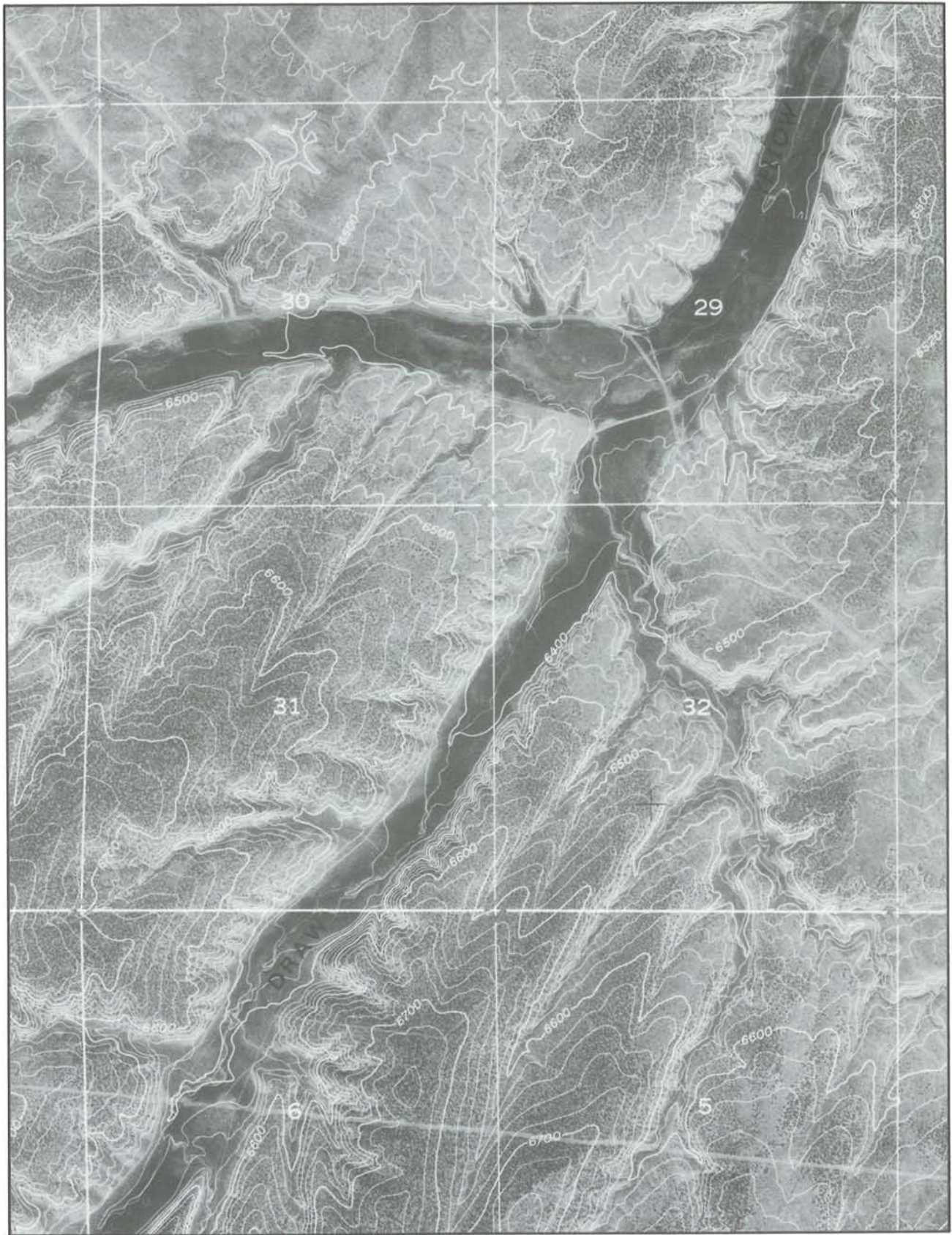
Figure 7. The U.S. Geological Survey 7.5-minute orthophoto map provides a corrected aerial photo with topographic and other map features.
