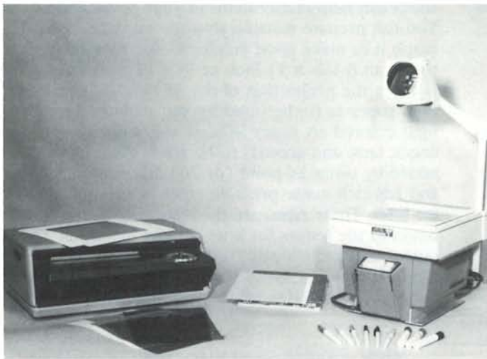
Equipment and materials used in making an overhead presentation. Left, a thermofax machine that transfers printed material onto transparencies. Center, transparencies that can be reproduced in a copying machine. Right, felt-tip markers for writing on acetate film, and an overhead projector.
