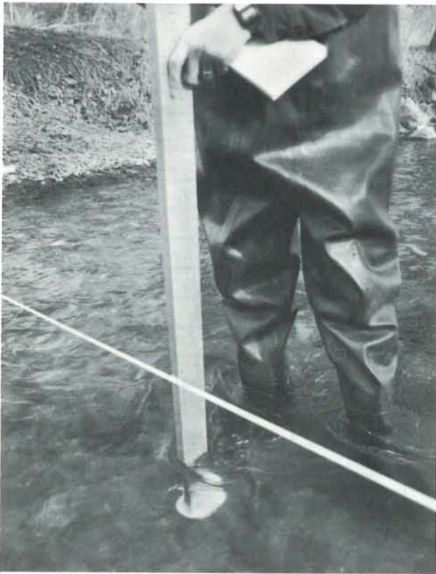
Figure 7. A velocity-head rod for measuring stream velocity.
