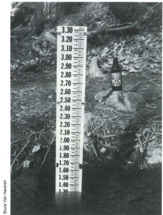
Figure 12. A staff gage for measuring water level.
