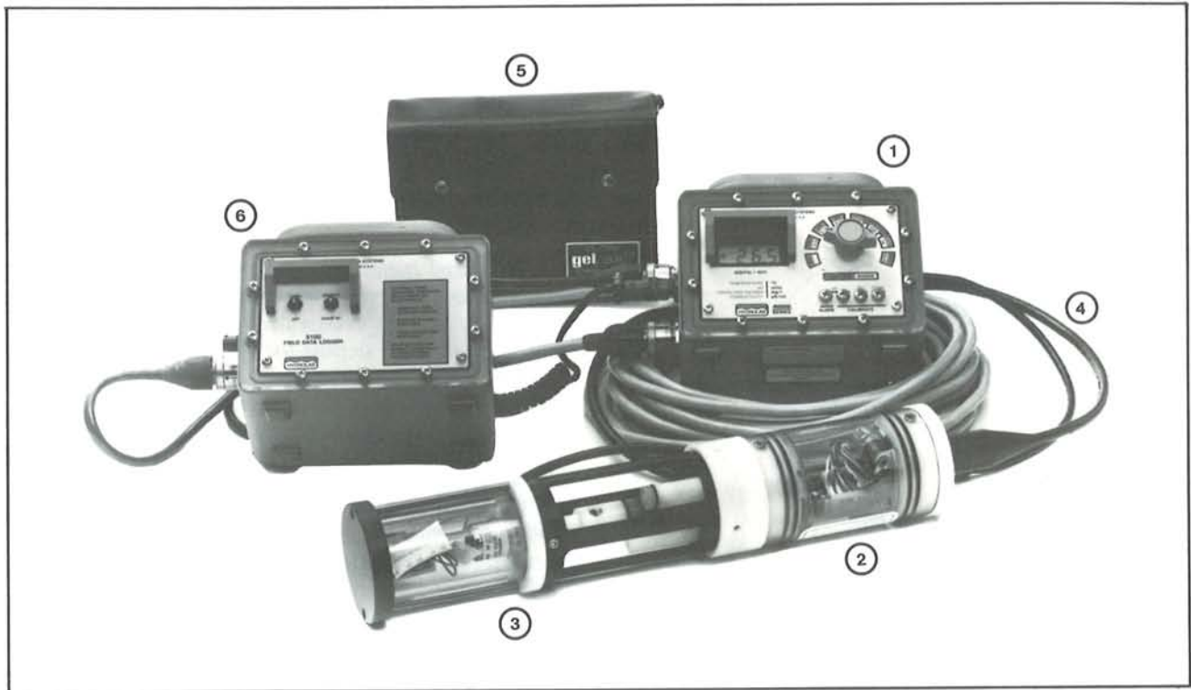
Figure 6. A multiparameter probe is used to measure profile data (courtesy of Hydrolab Corp.). (1) Digital Display Unit, (2) Sohle Unit, (3) Circulatory Assembly, (4) Cables, (5) Battery Pack, and (6) Digital Field Datalogger.
