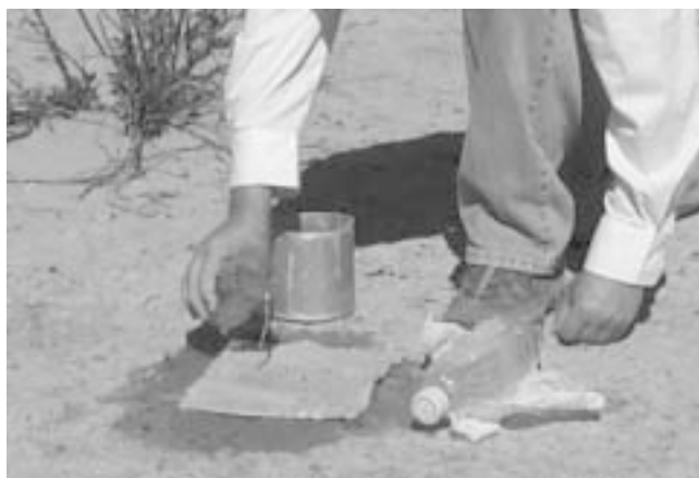
Figure 8.3. Pre-wet the soil to a 4 cm depth.
