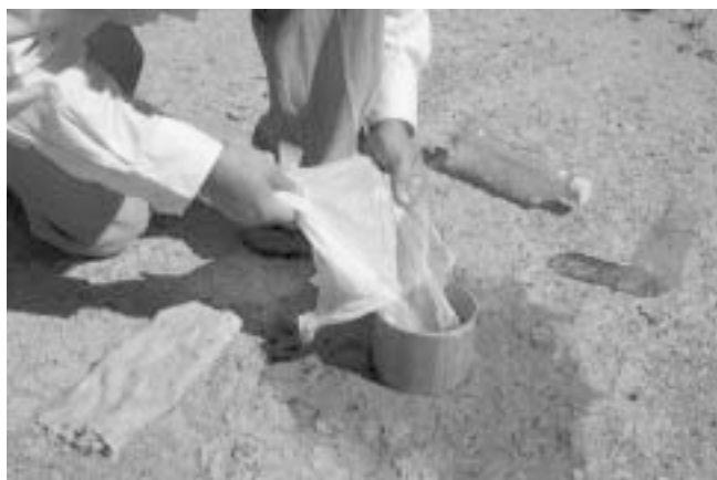
Figure 8.5. Add 370 ml water, using plastic sheet.
