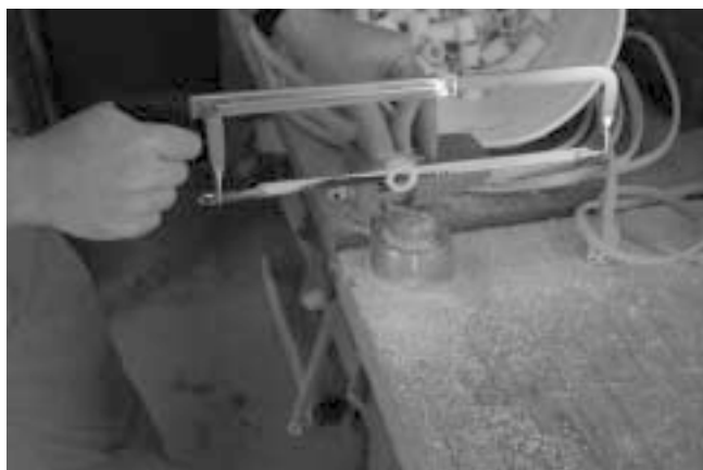
Figure A.1. First cut on PVC.
