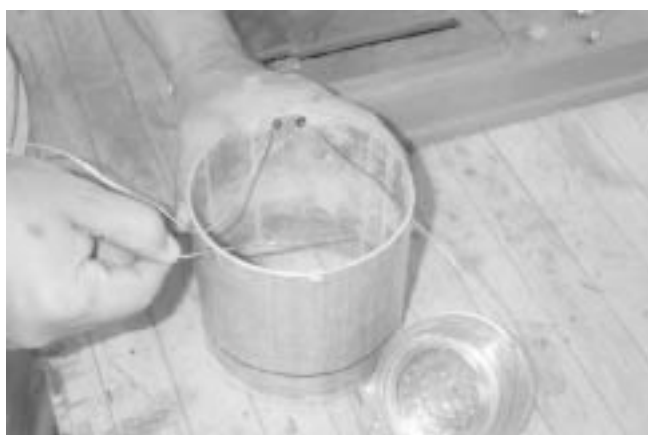
Figure A.8. Thread wire through holes and tighten.
