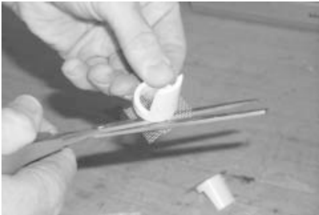
Figure A.4. Cutting out baskets from screen.
