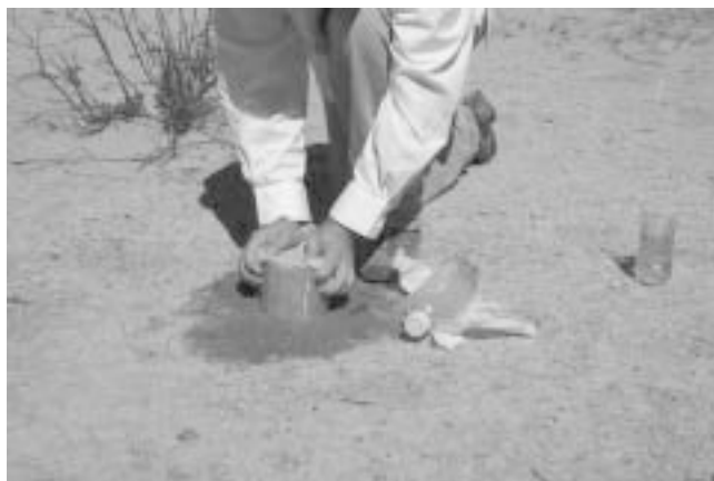
Figure 8.4. Insert infiltration ring to 3 cm.
