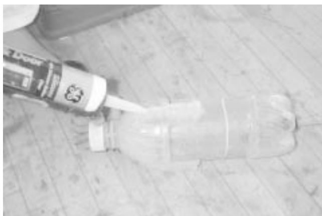
Figure A.10. Apply three 10 cm silicone beads from top of bottle to mid-section.
