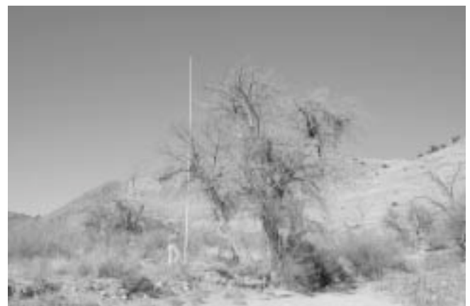
Figure 12.5. Measuring tree height with an extendable range pole.
