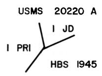
The X has been omitted from the inscription on bearing trees which is incorrect, unless the measurement was taken to the center of the tree. It should be included, thus: JD-1-20220A XBT or JD-1-PRI-1-20220A XBT if the full complement of marks are shown.
